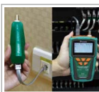
Verify LAN/ Telephone/ Coaxial cable condition
